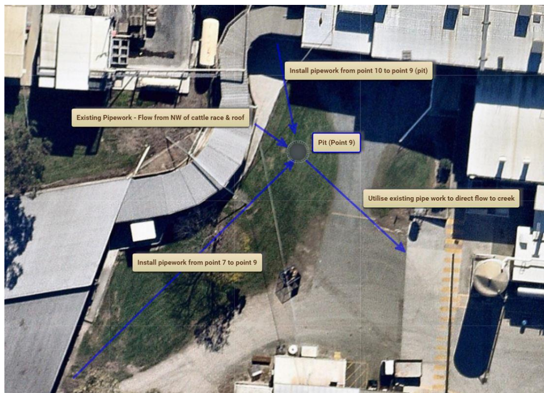
Figure 1 Proposed stormwater drainage upgrade
