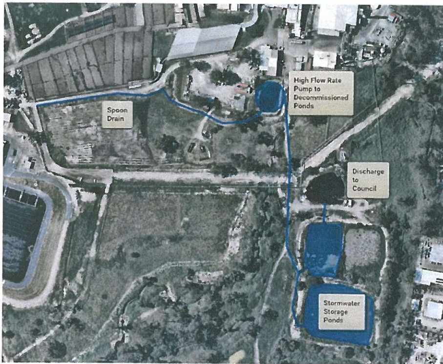
Eastern Stormwater Concept Design: Pumping from the Eastern Catchment Pond to the Stormwater storage ponds.
