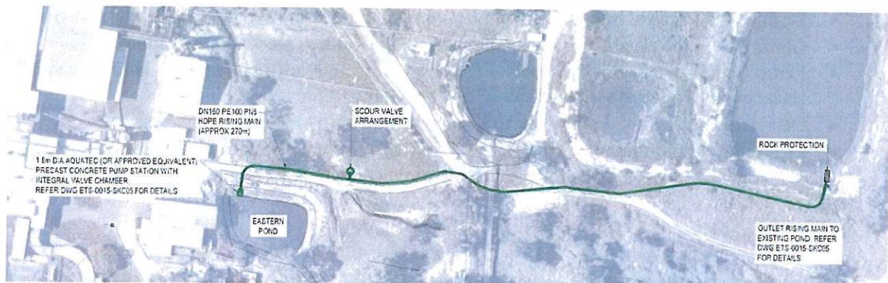
Figure 2 – Eastern Pond Pump Station and Rising Main
