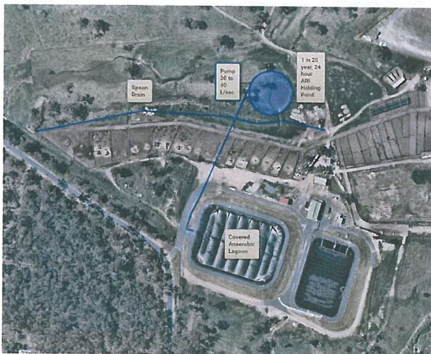
Western Catchment Stormwater Concept Design: Pumping from Western Catchment Pond to the CAL
