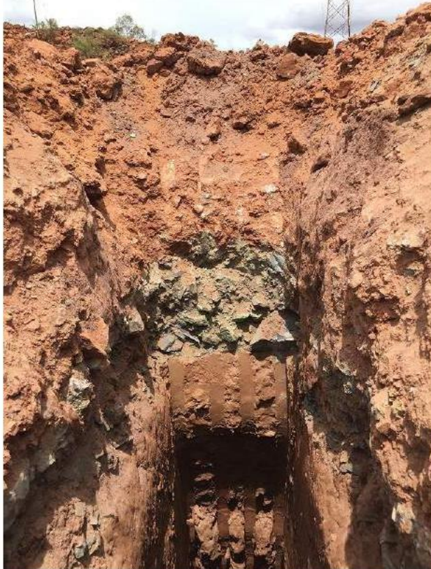
Photo 1 TP01 at Old TSF- note gravelly layer above tailings
