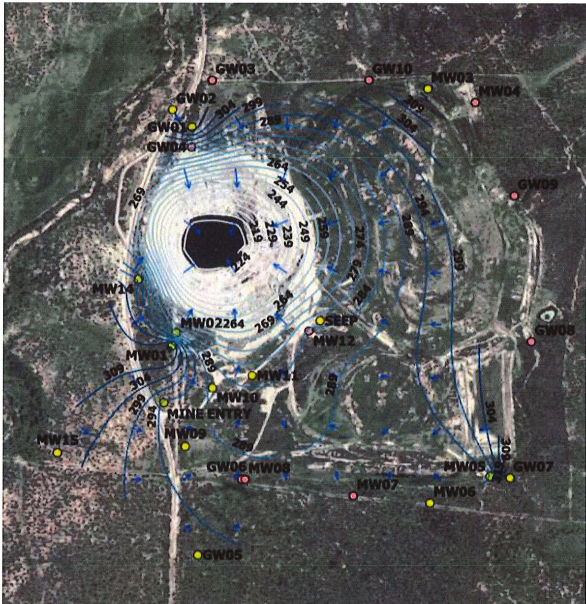
Figure 2.7 Fourth Quarter 2016 Groundwater Contour Map (Mining One 2017)
