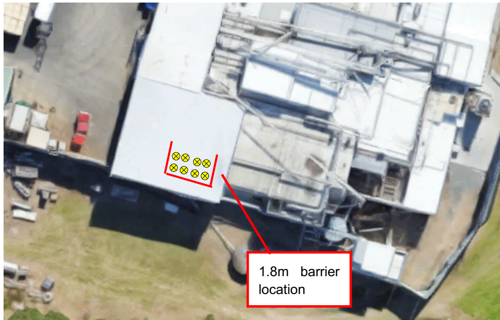
Figure 6-1 Odour Fan Barrier
