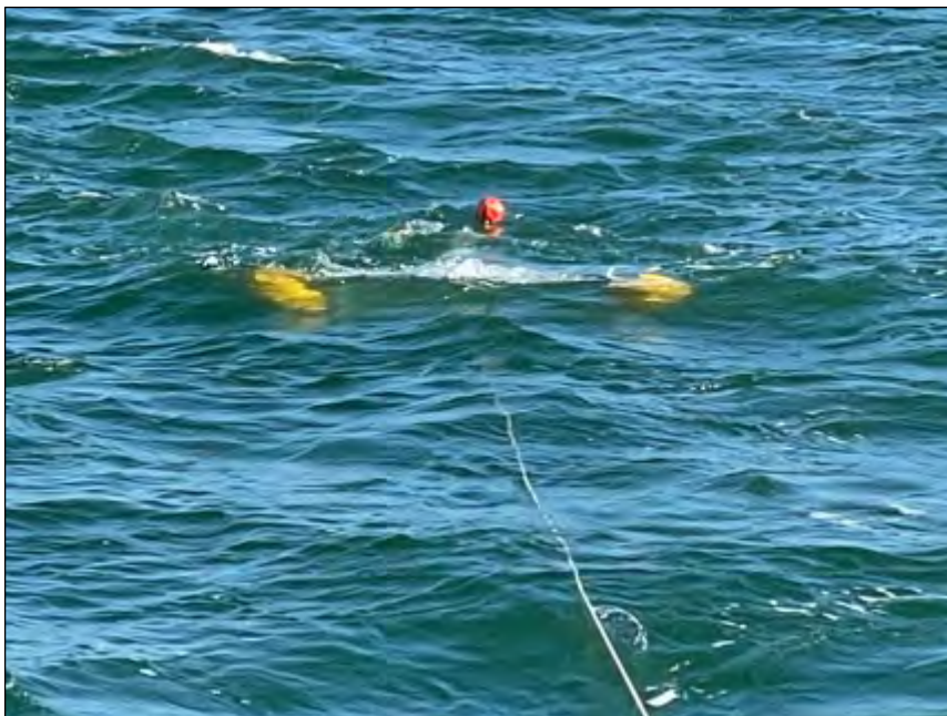
Figure 2.2 Manta trawl used to collect benthic biota (yellow floats were removed for benthic sampling).
