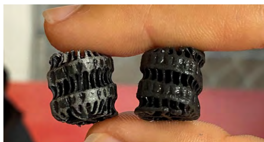
Figure 3 - Comparison of Edge Rounding of In-Service and Test Carrier
