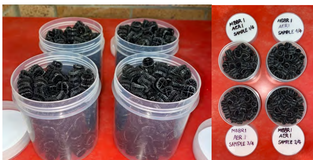
Figure 4: MBBR Carriers from Aeration Tank 1
