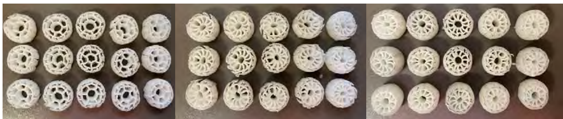
Figure 12 - Breakage of Bioflo+ (L), Biopipe (C), and Biotag (R) Carriers
