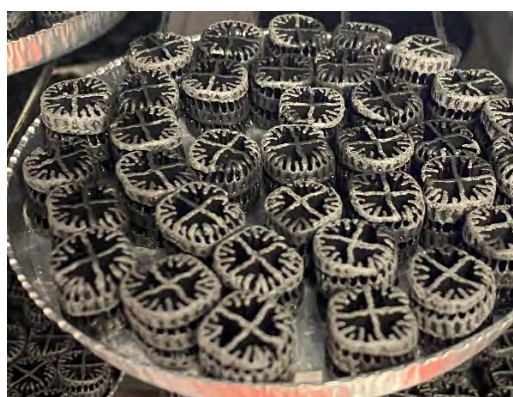
Figure 4 - Whitening Characteristic of In-Service Carriers
