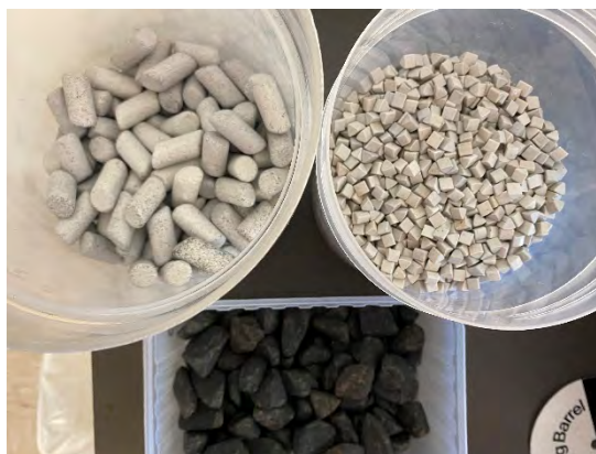
Figure 2 - Examples of Porcelain Ceramic and Blue Metal Grinding Media Types
