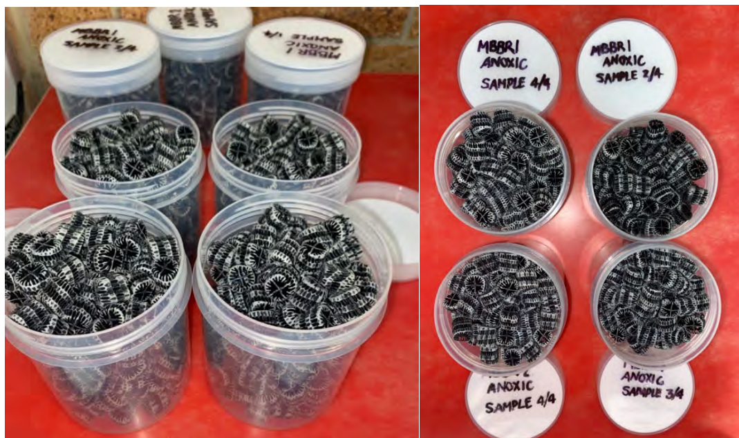
Figure 3: MBBR Carriers from Anoxic Tank
