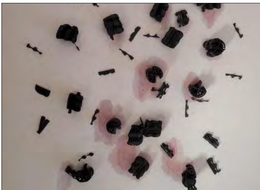
Figure 2.3 Broken down MBBR carriers.
