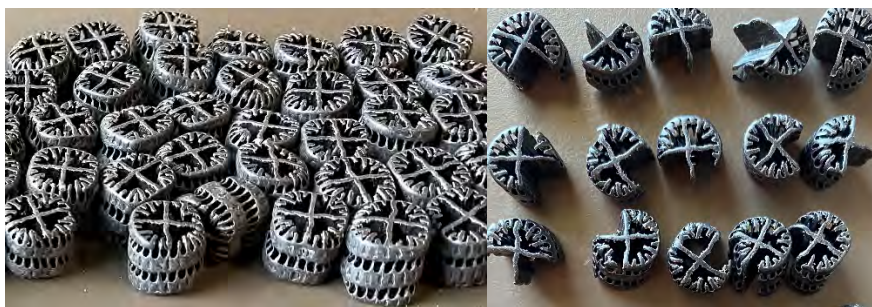
Figure 8 - Characterisation of Carrier Degradation Mechanisms: Wear (L) and Breakage (R)
