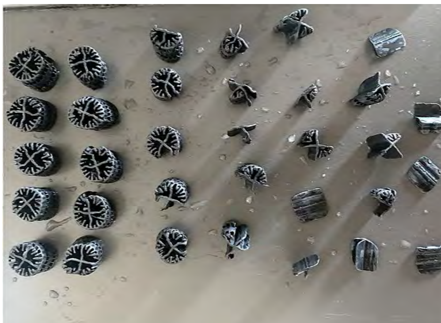
Figure 9 – Degradation of Hel-X Carriers Throughout Rotary Tumbler Test (L to R: progressive through test)
