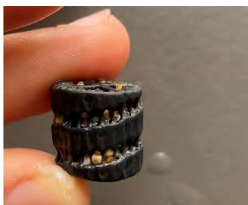
Figure 5 - Coarse Sand Grinding Media Trapped in Carrier
