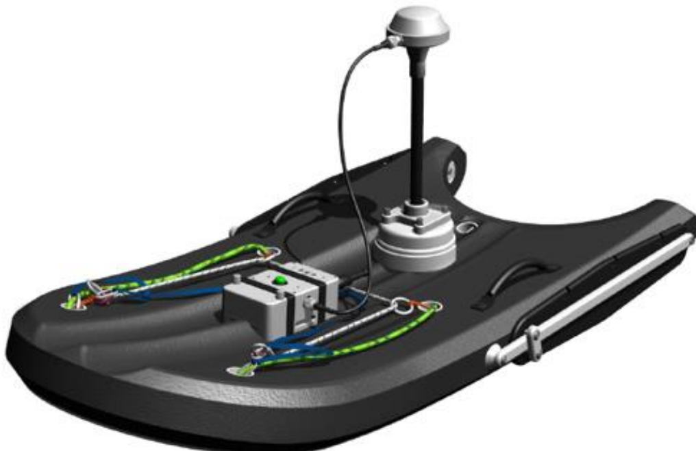
FIGURE 6-3 M9 UNIT (UPPER) AND M9 PLACED IN THE HYDROBOARD (SOURCE: SONTEK 2018)
