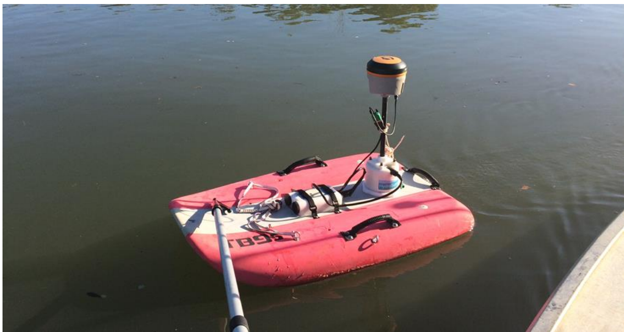
FIGURE 8-3 DOWNWARD FACING ADCP MOUNTED ON AN UNMANNED VESSEL AND TOWED ALONGSIDE A FIELD BOAT
