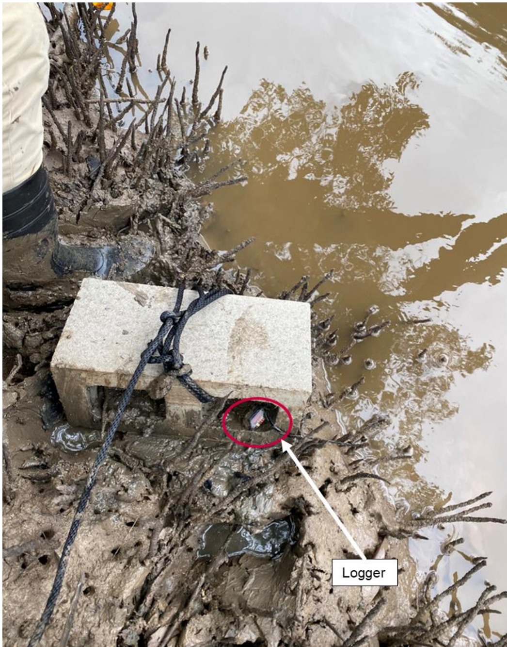
FIGURE 6-6 WATER LEVEL LOGGER MOUNTED ONTO BESSER BRICK
