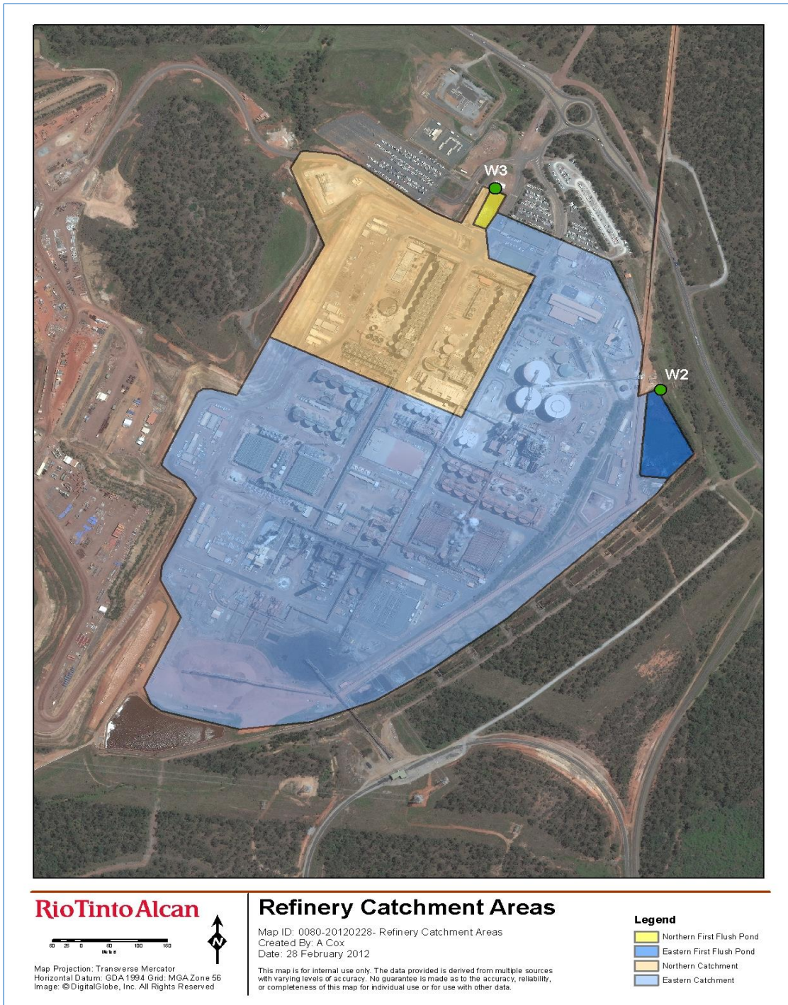
Figure 1 - Refinery Catchment Areas – First Flush Catchment
