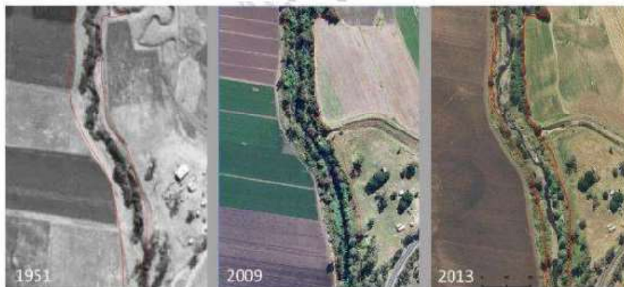
Figure 2: Laidley Creek bank alignment in Reach 1 from 1951 to 2013 – the red lines indicate top of macro-channel bank in 2013
