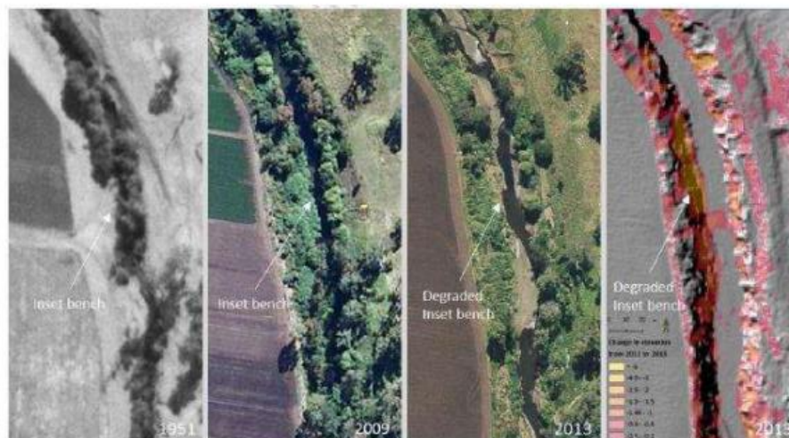
Figure 3: Degradation of inset bench within Reach 1 Laidley Creek demonstrated by change in aerial photography and change in elevation between 2011 and 2013 displayed on 2014 LIDAR (yellow and pink displays a drop in elevation indicating erosion has occurred)
