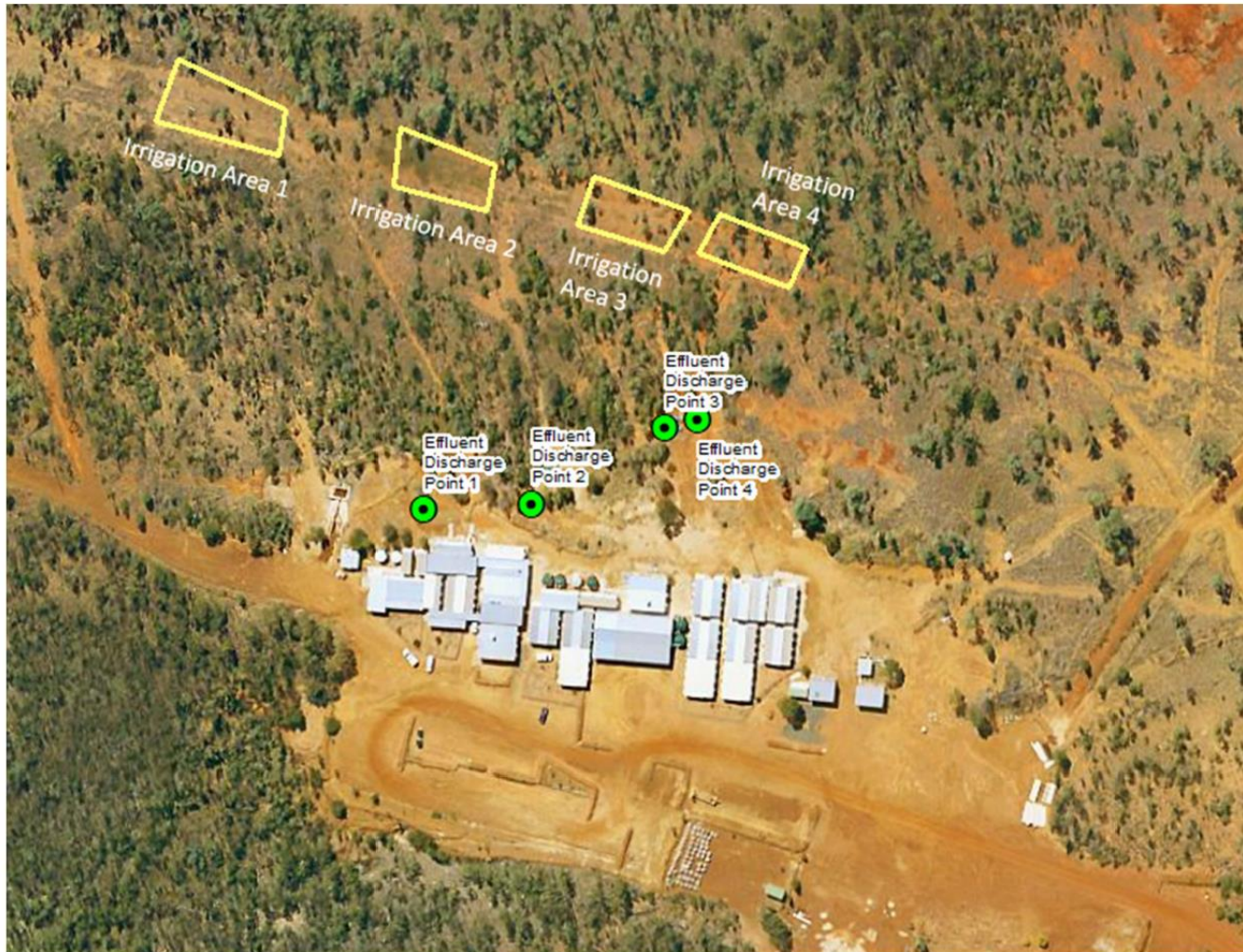
Figure 4: Irrigation areas and effluent discharge points
