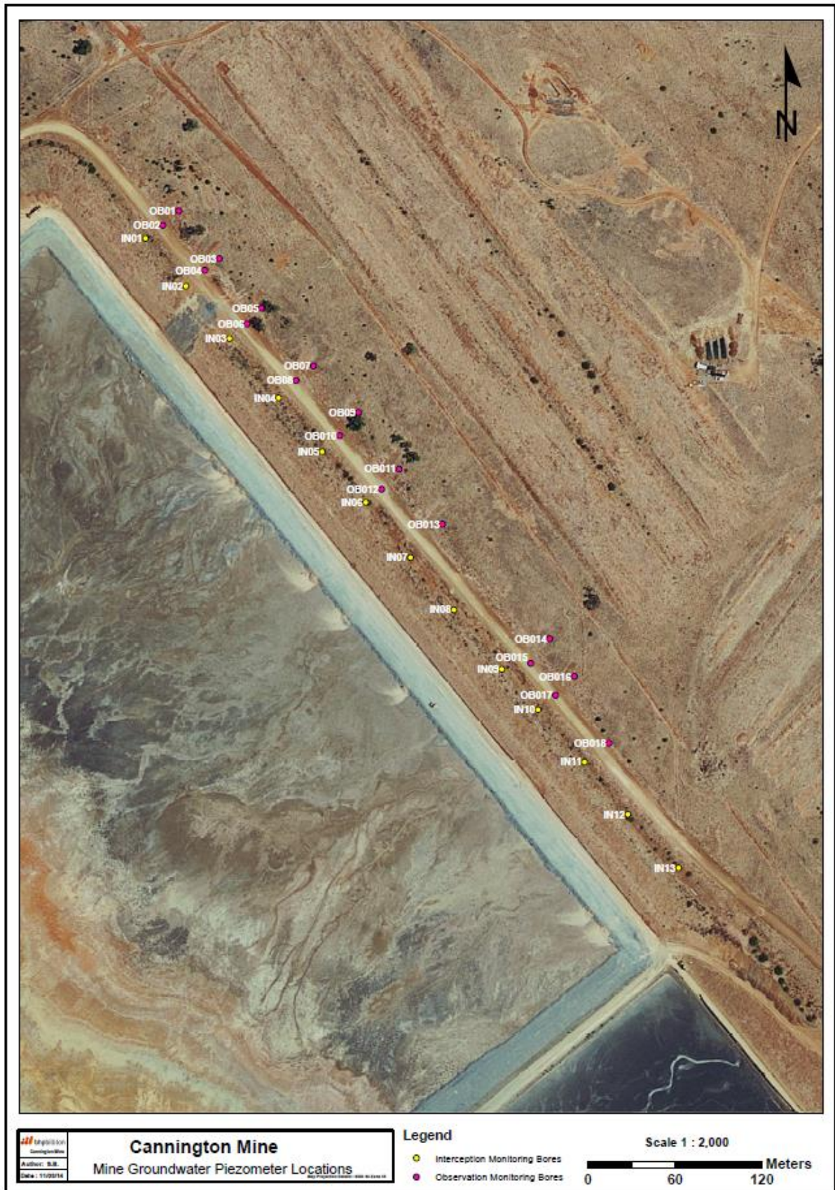
Schedule J – Figure 12 (TSF Seepage Monitoring Locations A)
