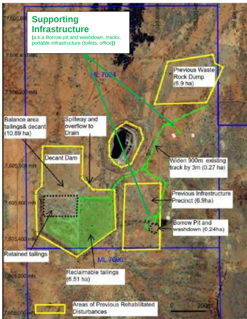
Figure 1b: Project Infrastructure Layout – Supporting Infrastructure
