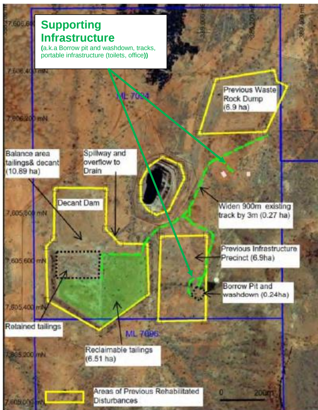
Figure 1b: Project Infrastructure Layout – Supporting Infrastructure
