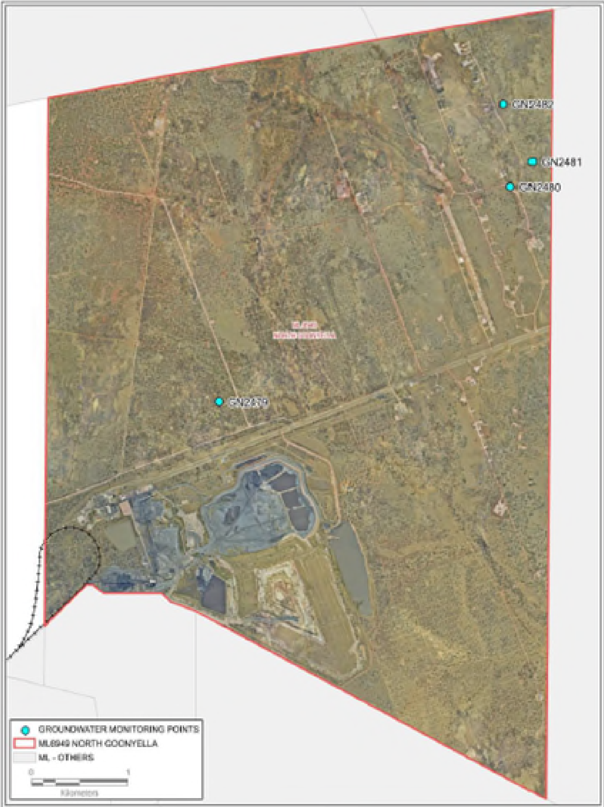
Figure 3 – Groundwater Monitoring Locations
