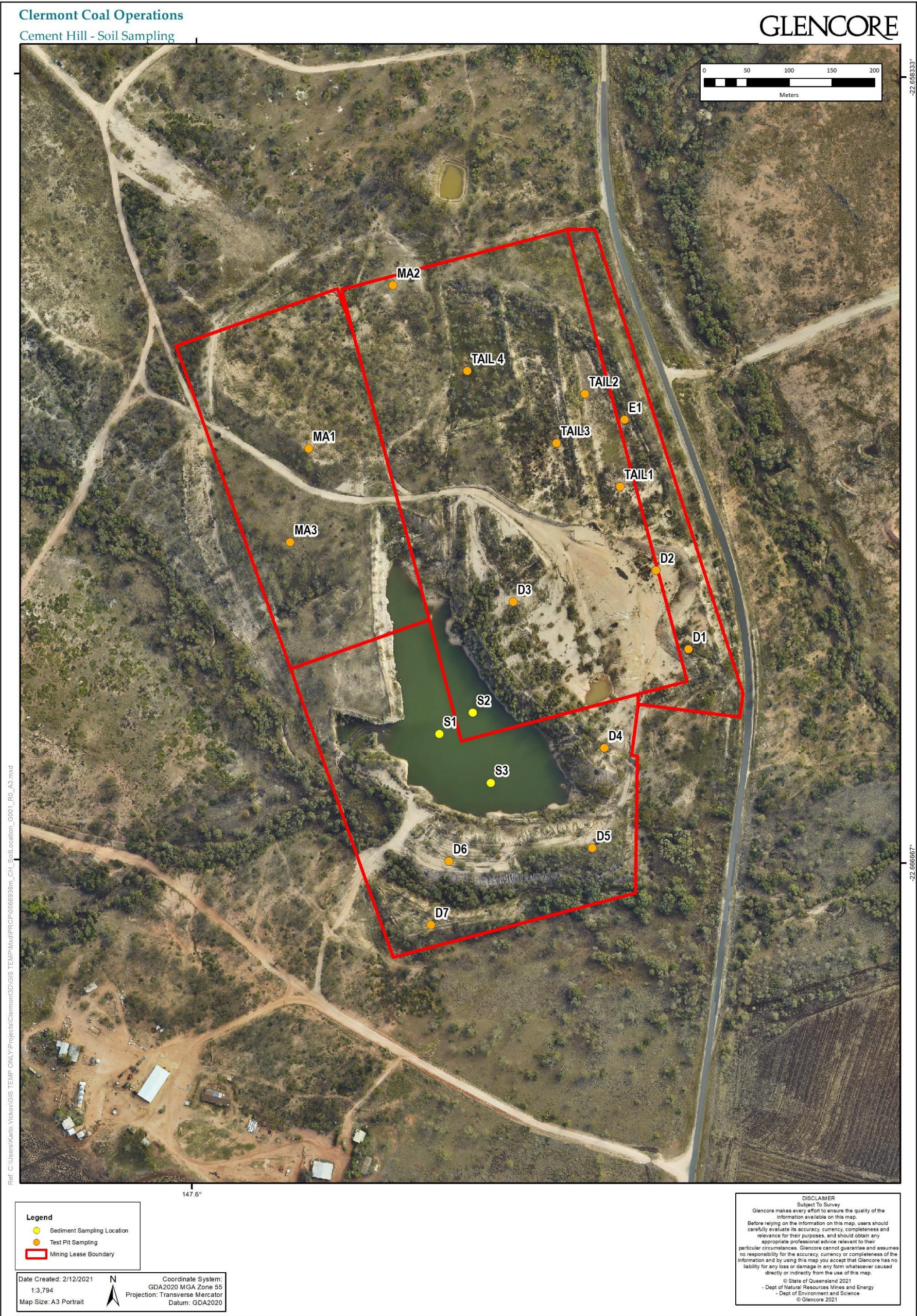
Figure 3-1 - Location of soil test pits
