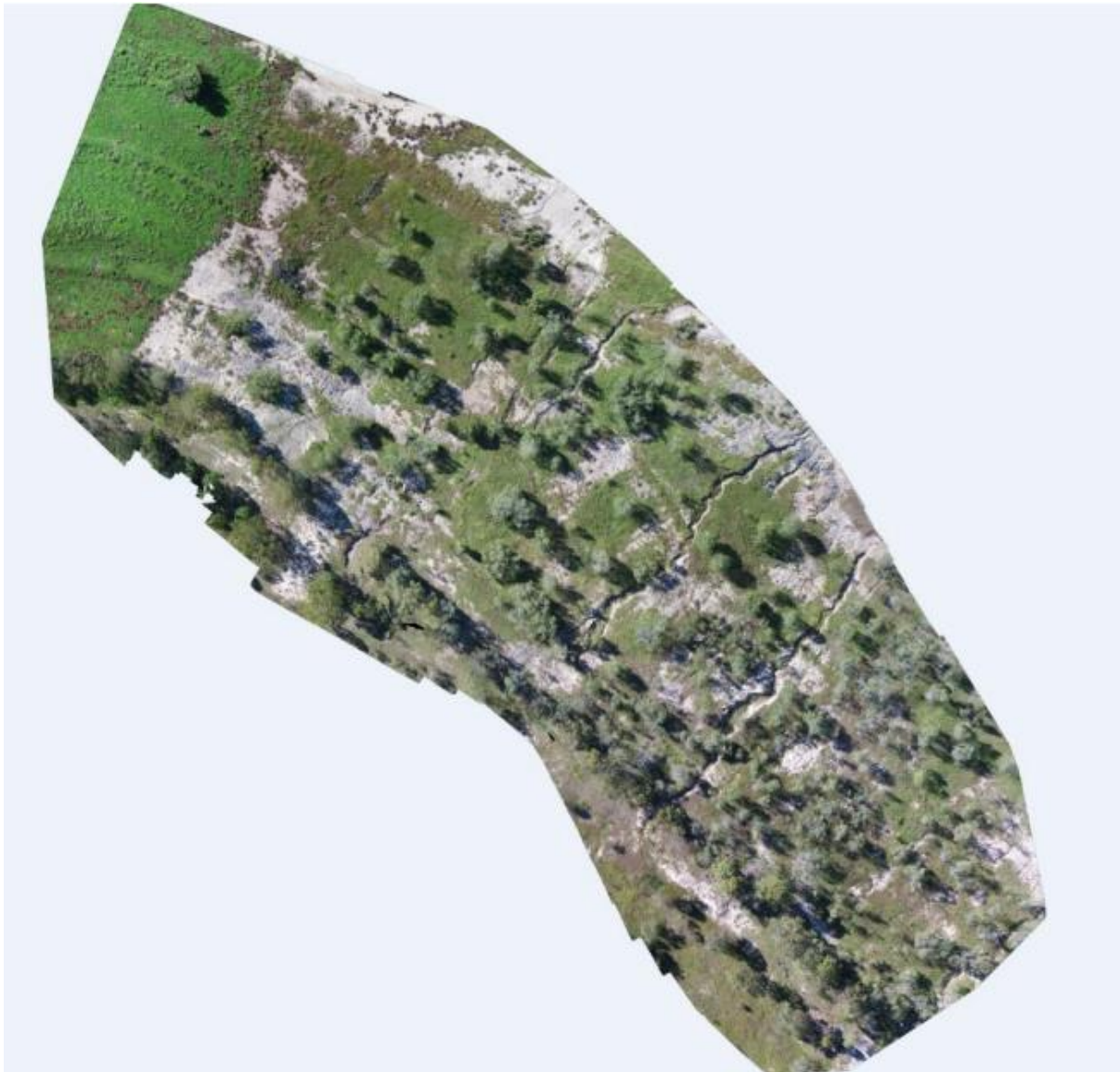
APPENDIX 2 - IMAGE 6: SHEET AND CHANNEL EROSION ON OPD NORTH-EASTERN BATTER SLOPE
