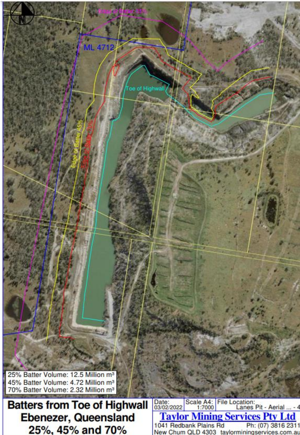
APPENDIX 5 - PLAN 37: HIGH-WALL CREST AT 25%, 45% AND 70% SLOPE
