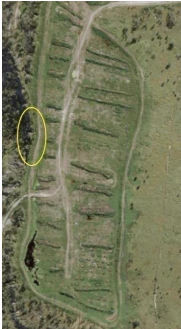
IMAGE 28: LOCATION OF SLIPPAGE ON WESTERN EDGE OF COMPOST PAD
