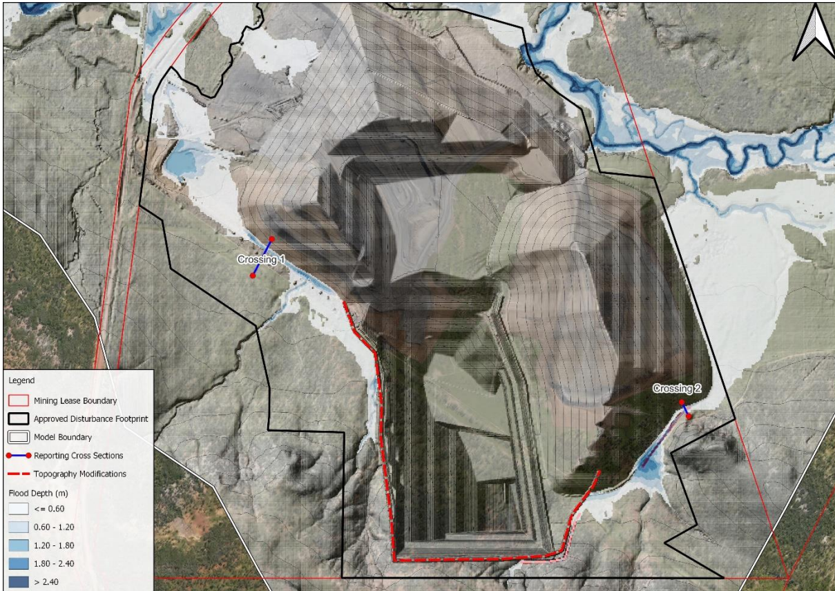
Figure 5.1: 0.1pct Flood Depth Around Final Landform
