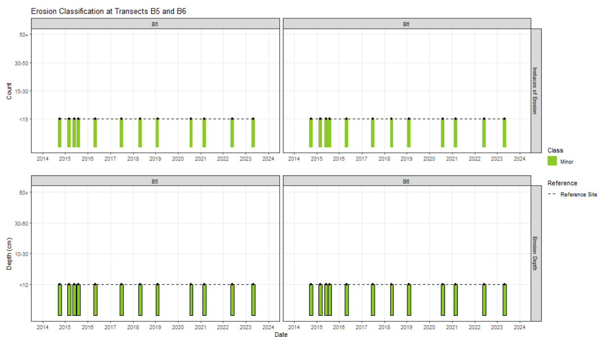
Figure 4-45: Erosion within Cell B thin (B5) and thick (B6) gravelly topsoil capping trial
