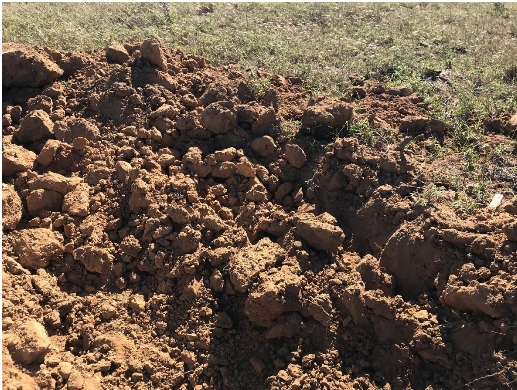
Figure 3.5: Test Pit 1, off-site clay borrow material.
