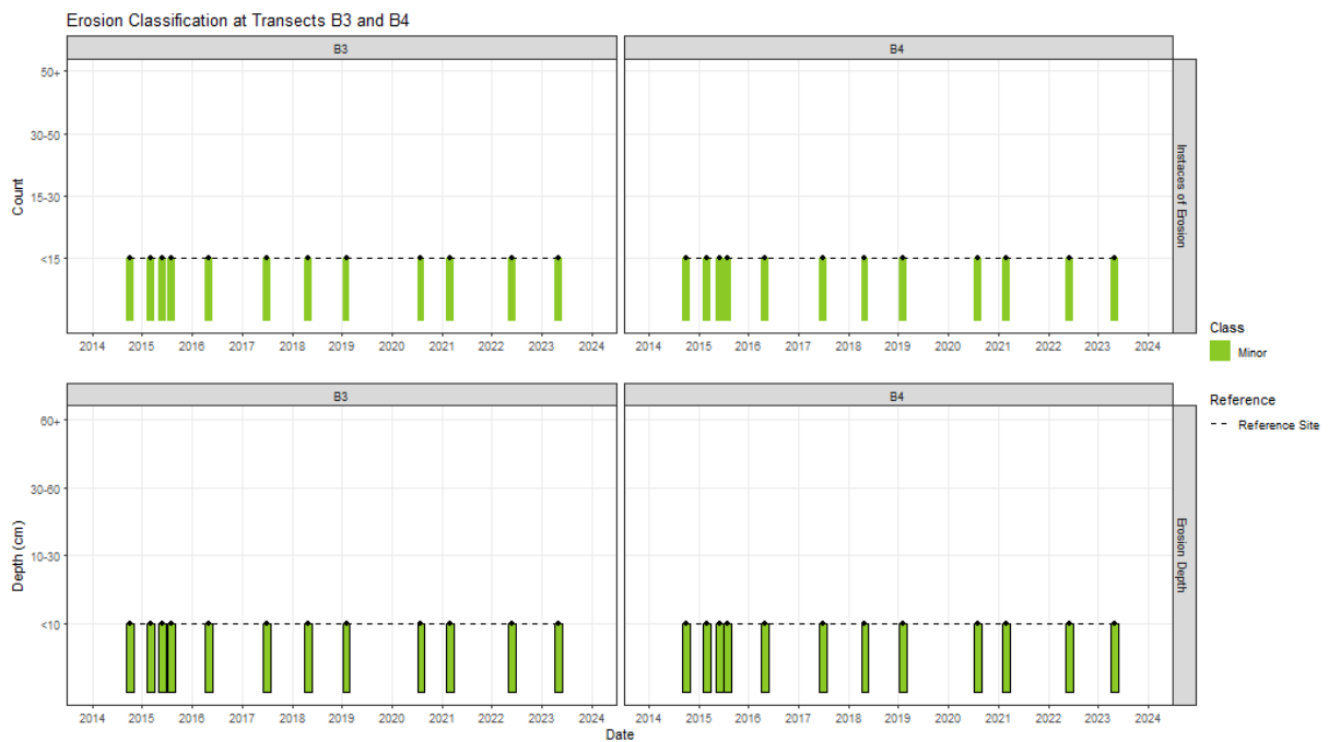
Figure 4-40: Erosion categories for TSF Cell B thick topsoil cover trial (B3 and B4)
