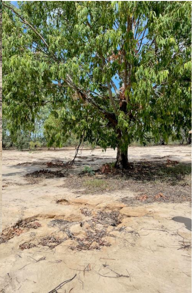
Figure 47 - Views of differential settling & internal erosion visible on the tailings surface
