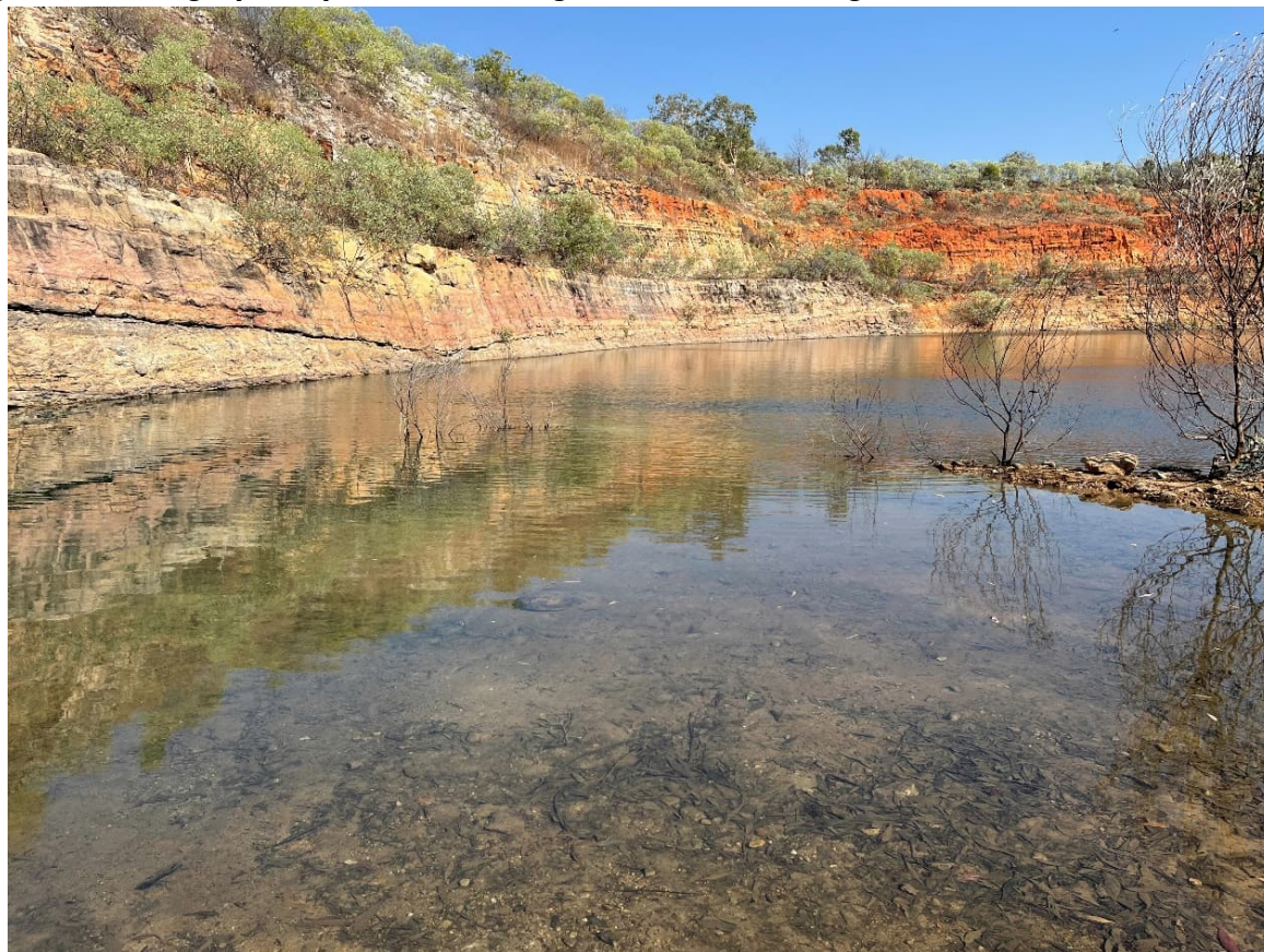
Figure 9 Photograph of pit wall showing horizontal bedding
