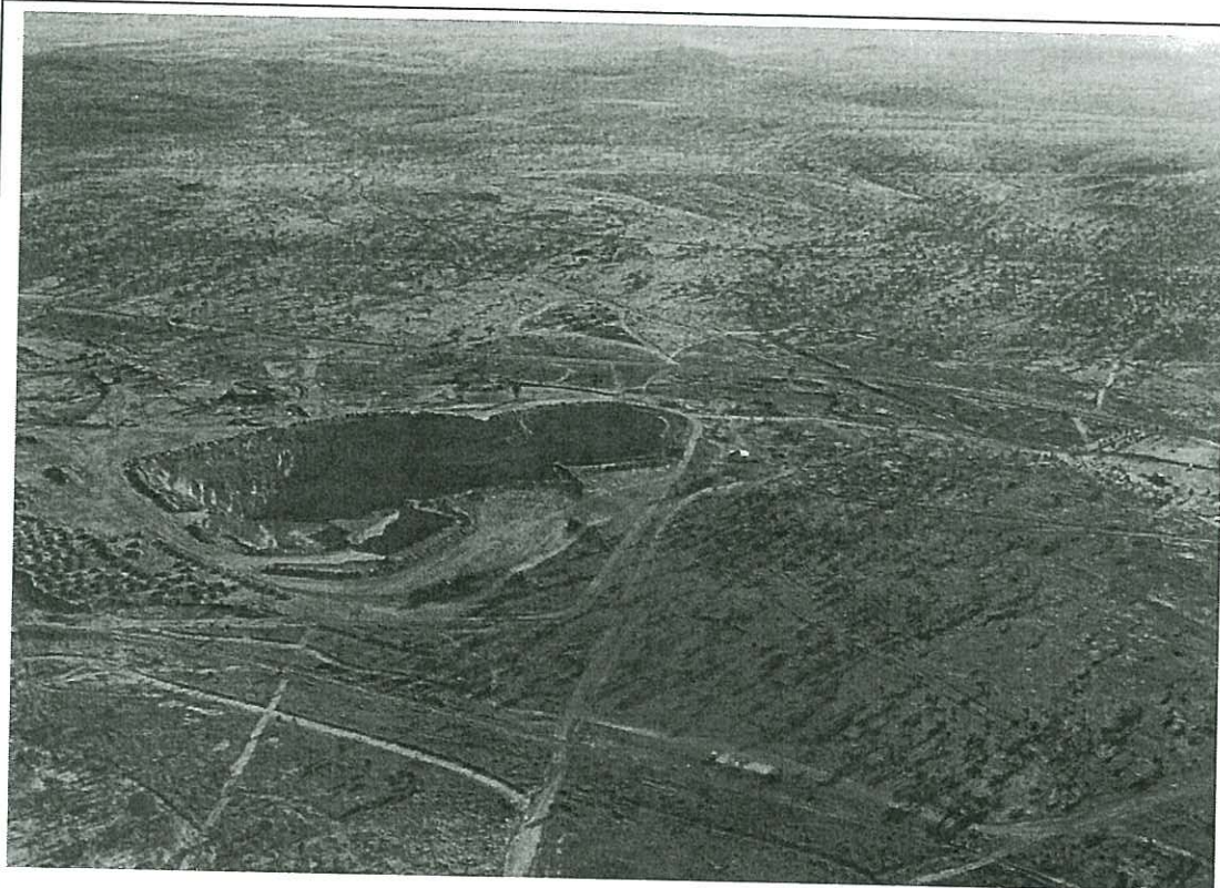
Aerial view of Golden Butterfly pit with 10 metres depth to go. Note hardstand area on left with ore stockpiles. October 1989.
