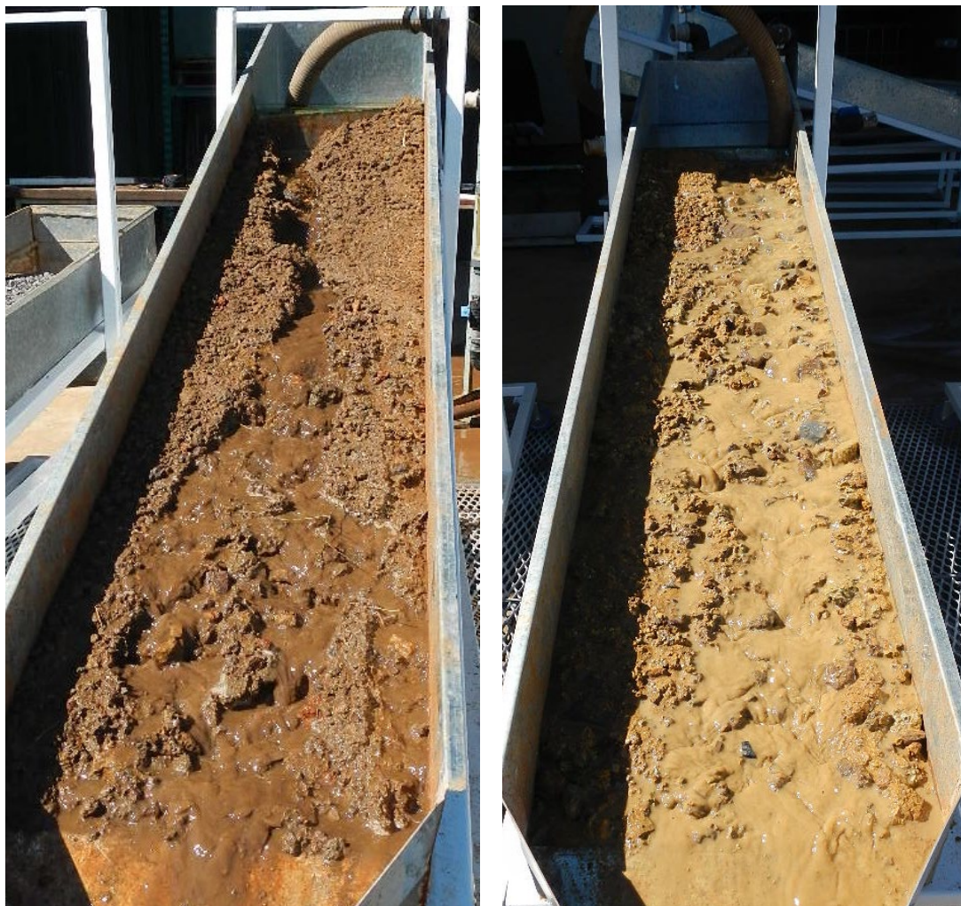
Figure 1: Flumes showing application of flow to D1 (topsoil) (left) & D3 (tertiary) (right) samples.
