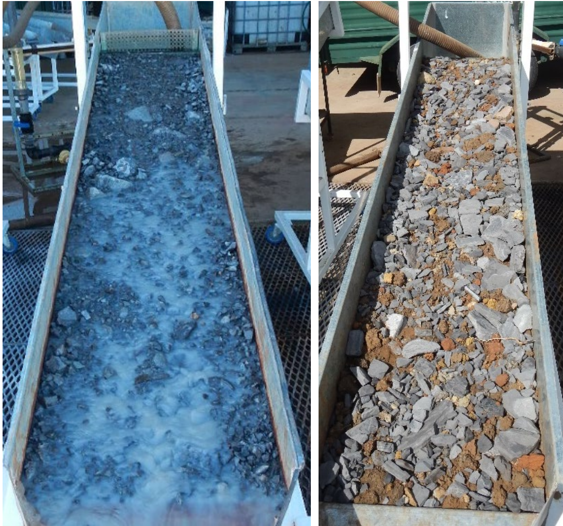
Figure 2: Flumes of Permian waste rock (left) (sample D6), showing surface flow developing on the lower half of the plot only, and of waste rock (D5) mixed with topsoil (D1) (right) prior to application of flow.
