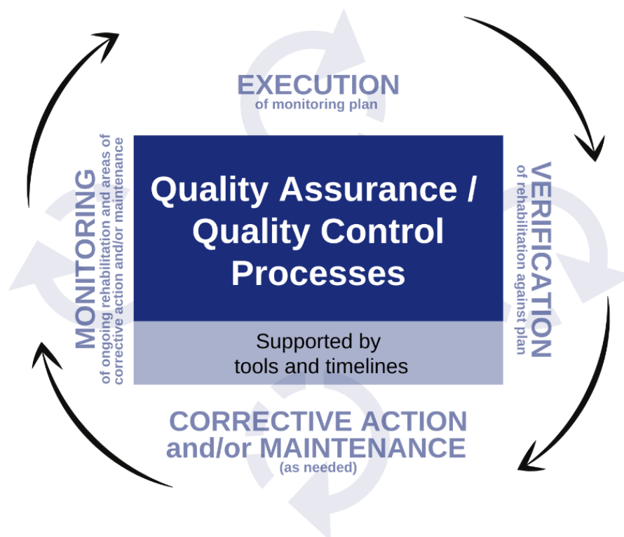
Figure 21: Rehabilitation monitoring quality assurance / quality control process
