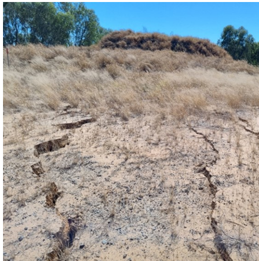
Longwall centreline – blocks move downwards (and to a lesser degree sideways) at discrete intervals
