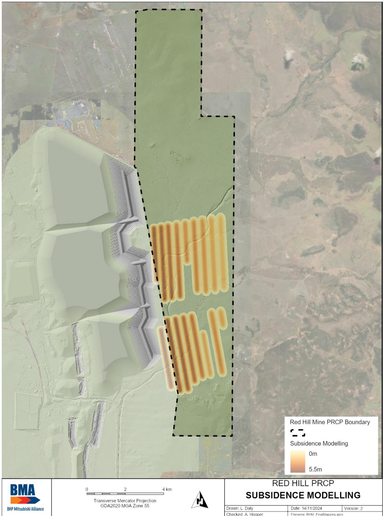
Figure 17: RHM modelled subsidence
