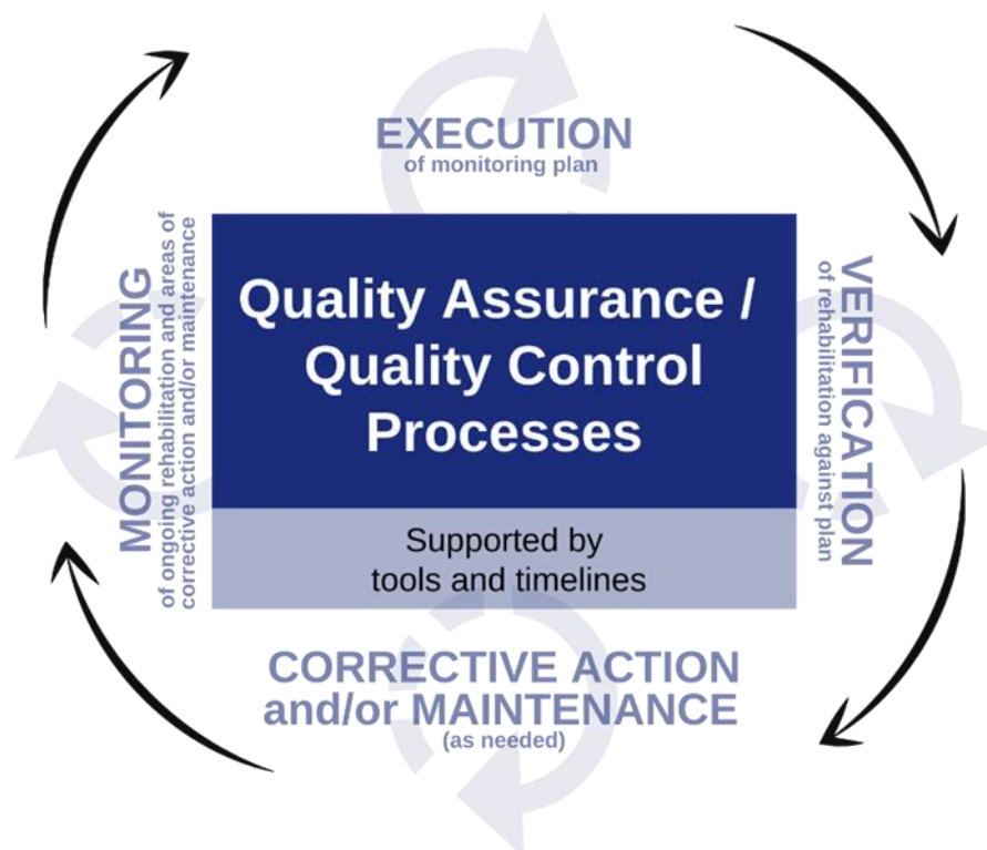
Figure 21: Rehabilitation monitoring quality assurance / quality control process
