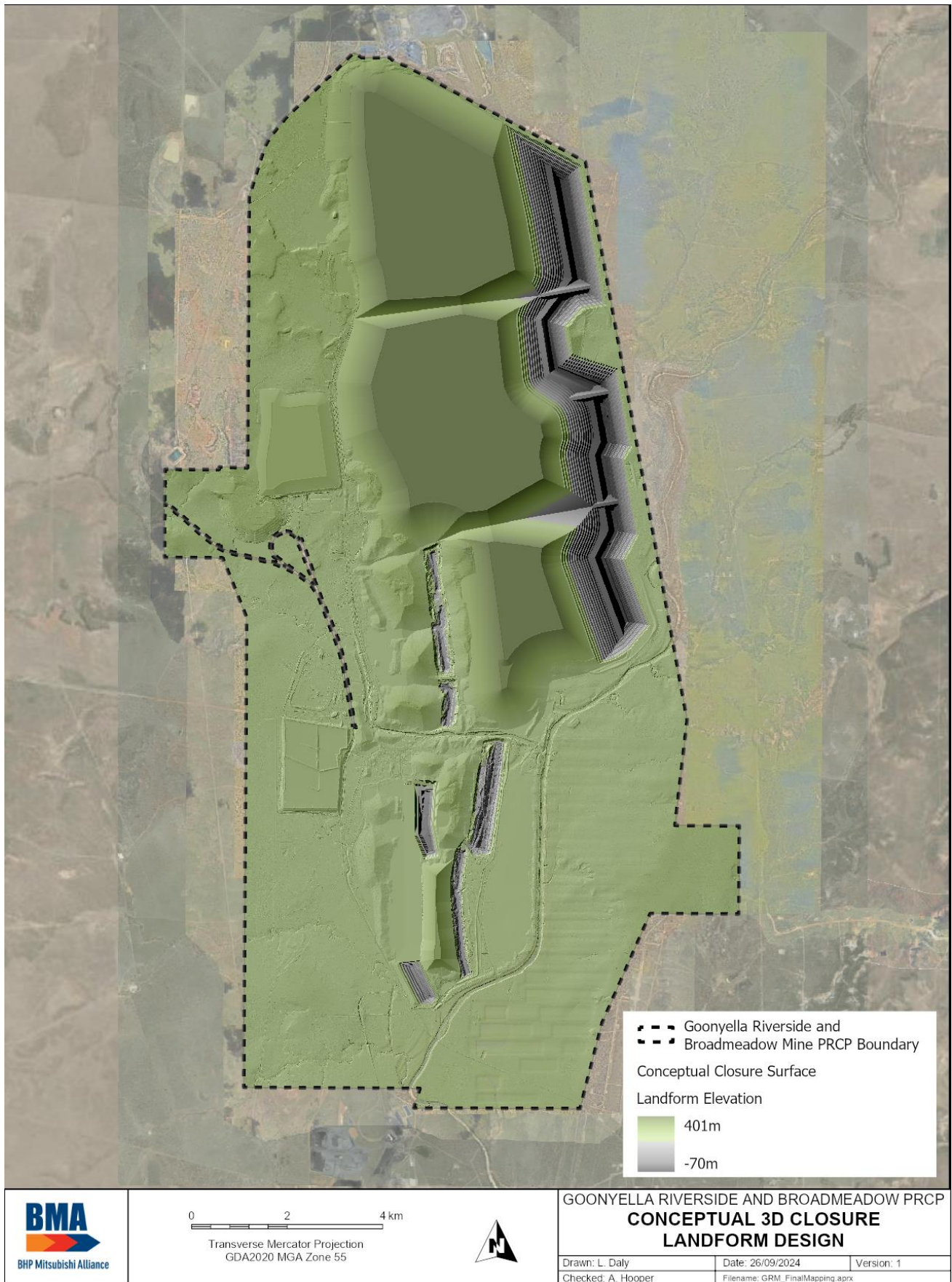
Figure 17: Conceptual 3D GRM and BRM closure landform design
