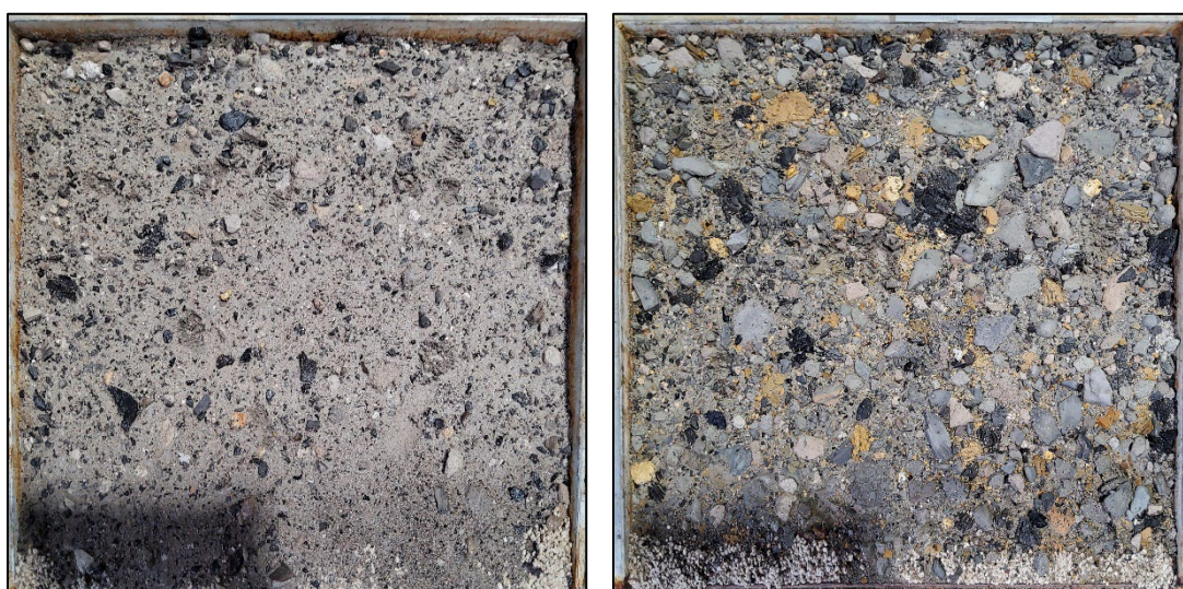
Figure 2: Test plots immediately following application of simulated rain to a Permian waste. R14_002 (left) and AH003_02 (right).
