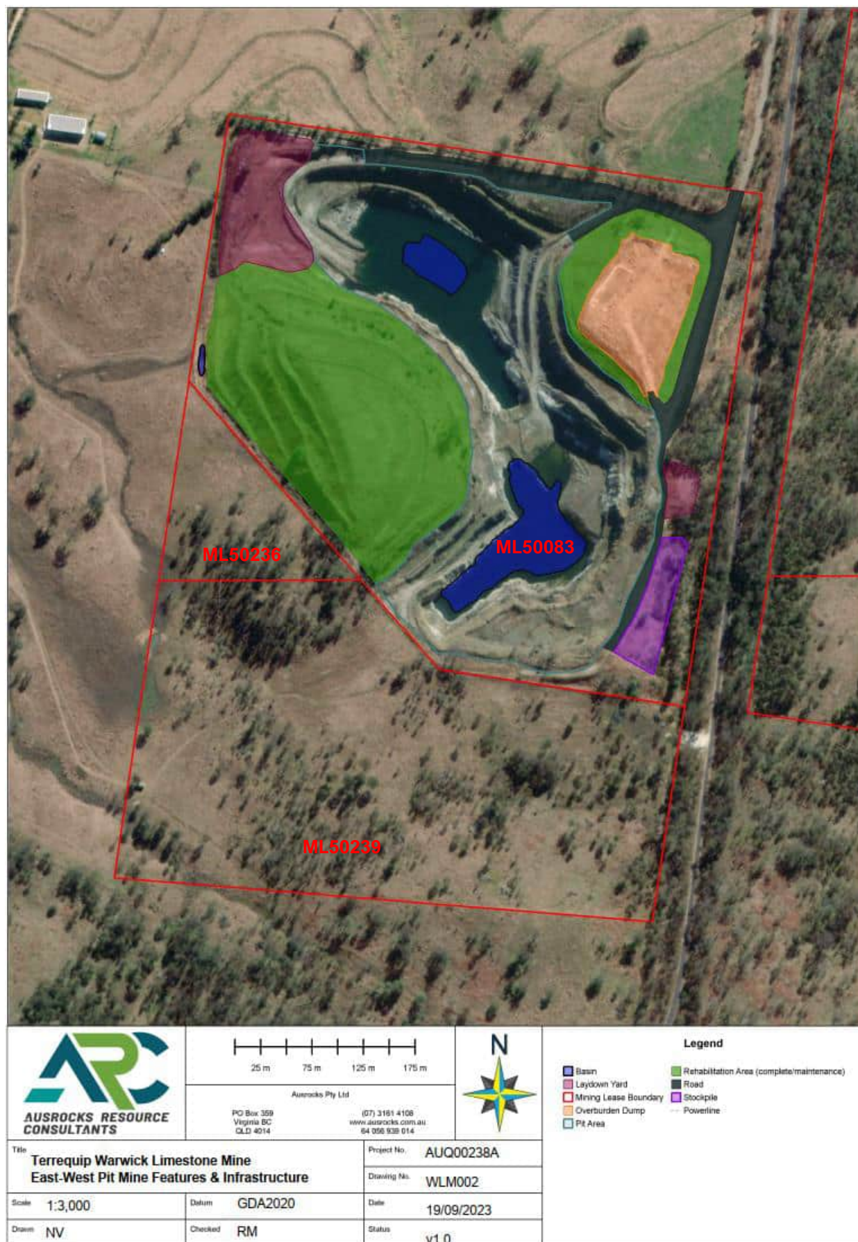
Figure 3: East-West pit mining tenements including primary mine features and infrastructure
