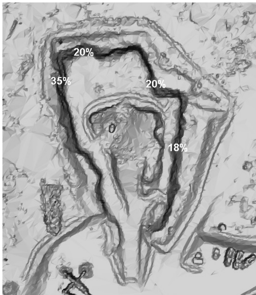
Figure 22. Upper bound overall scale stabilities (PoFs) around the Aspinall pit.
