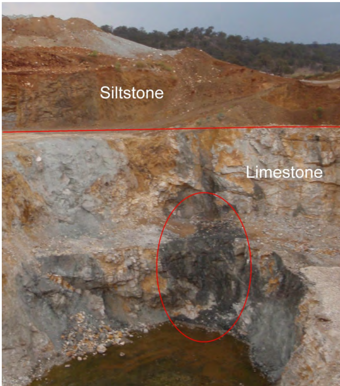
Figure 9. Limestone intruded by grey andesite exposed in the west wall at the north end of the East-West pit.
