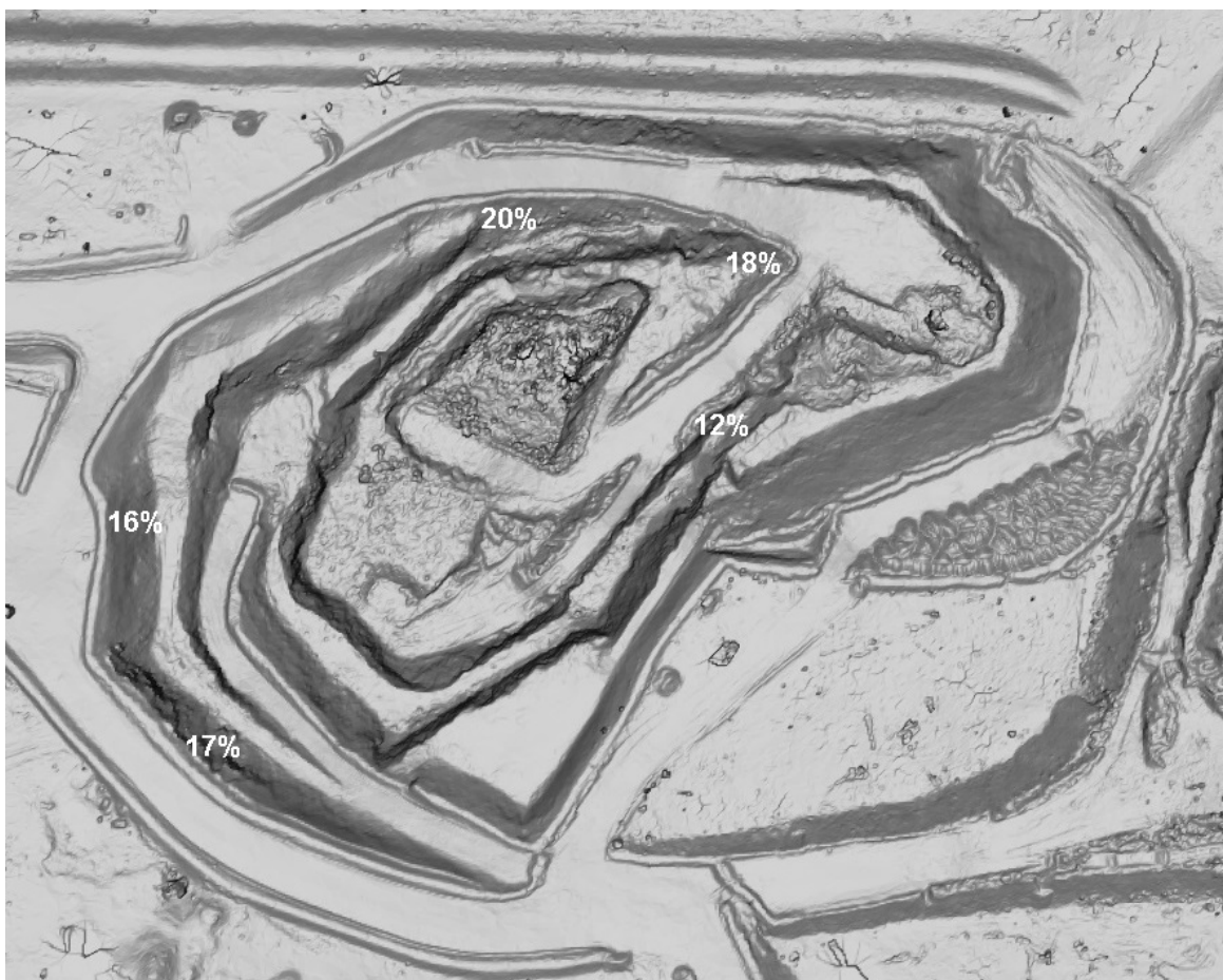
Figure 20. Upper bound overall scale stabilities around (PoFs) the Phoenix pit.
