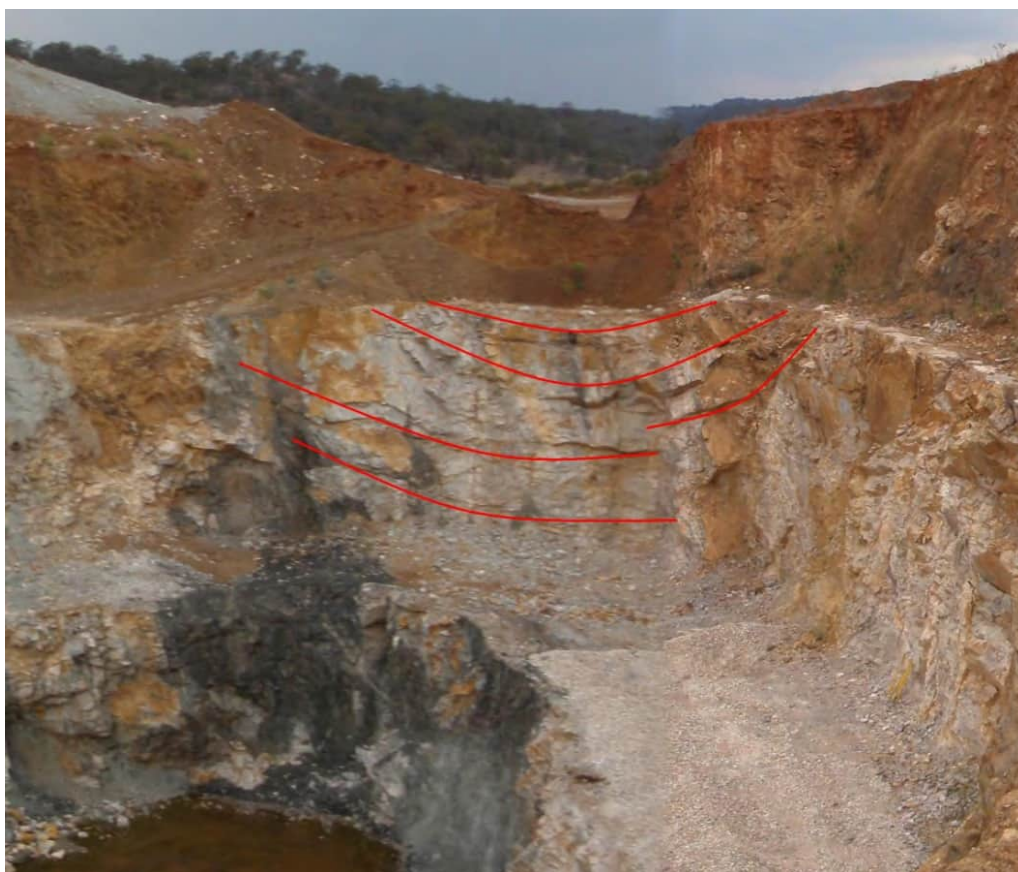
Figure 10. Example of synclinal fold in the upper benches at the west end of the East-West pit.
