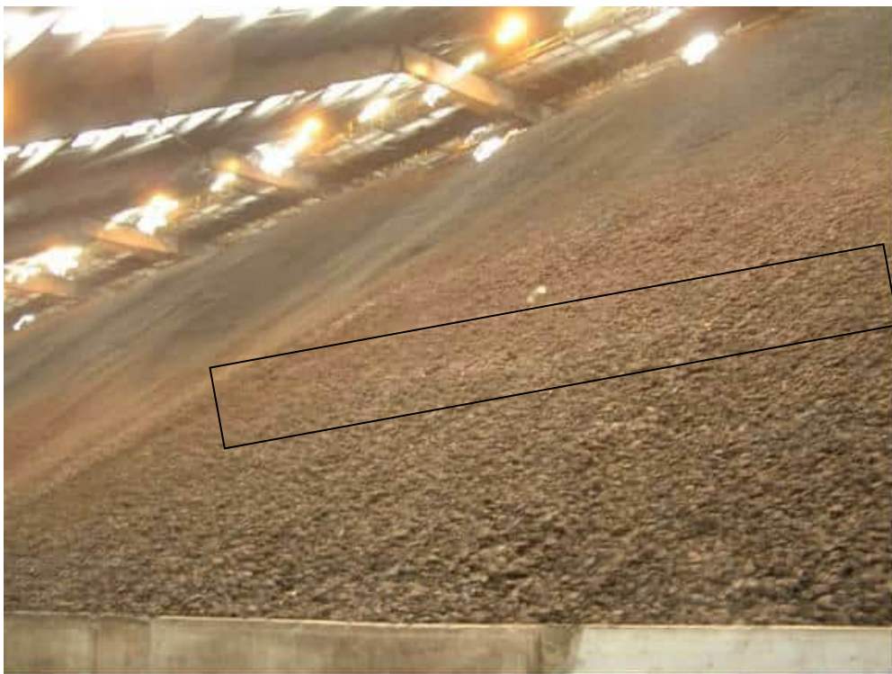
Figure 3. Enclosed stockpile storage of Kideco coal showing no compaction except from the weight of the stockpile and steep sides at angle of repose with coarse coal fraction accumulated at the base of the stockpile allowing pathways for air to enter the stockpile and create a chimney effect. Note the moisture condensation lines within the rectangular zone arising from hot spot development inside the pile. Thermal runaway reached in 10-13 days.
