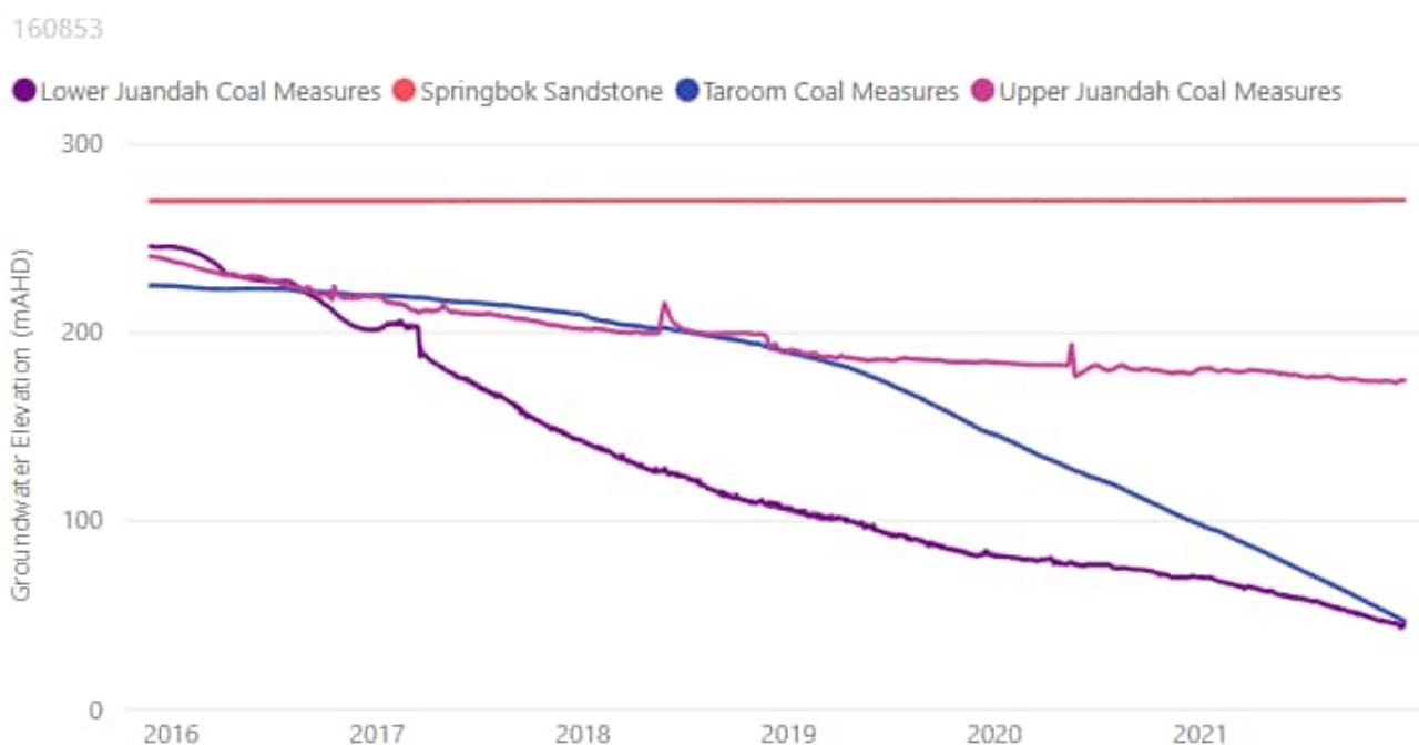
Figure 4.12 RN160853 Groundwater Elevation
