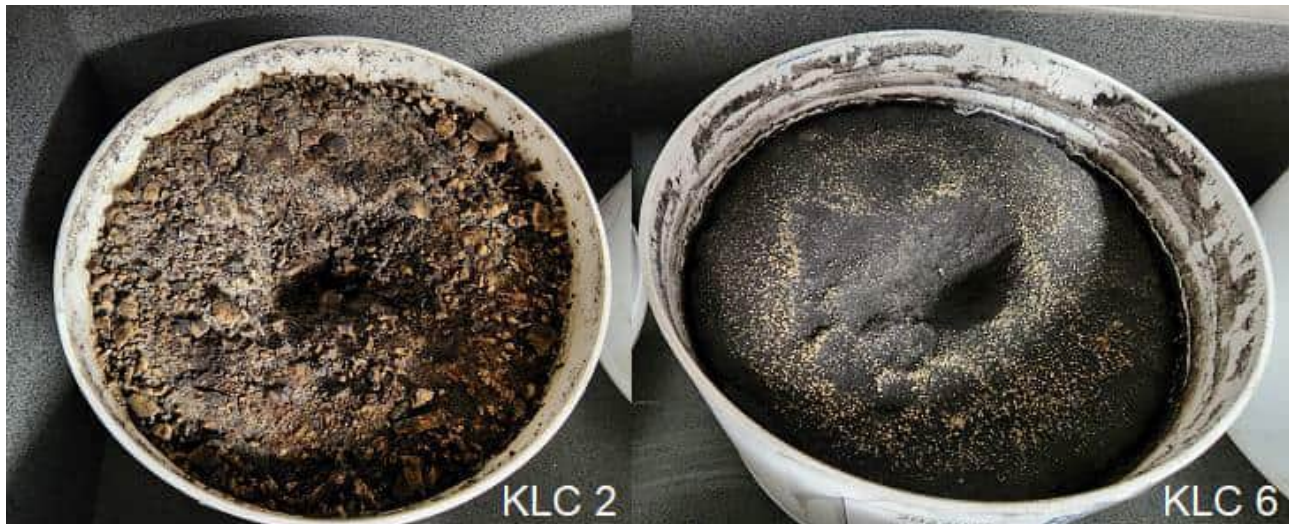
Figure 3-21: Secondary mineral formation on low quality/grade coal (WS1A) and tailings
