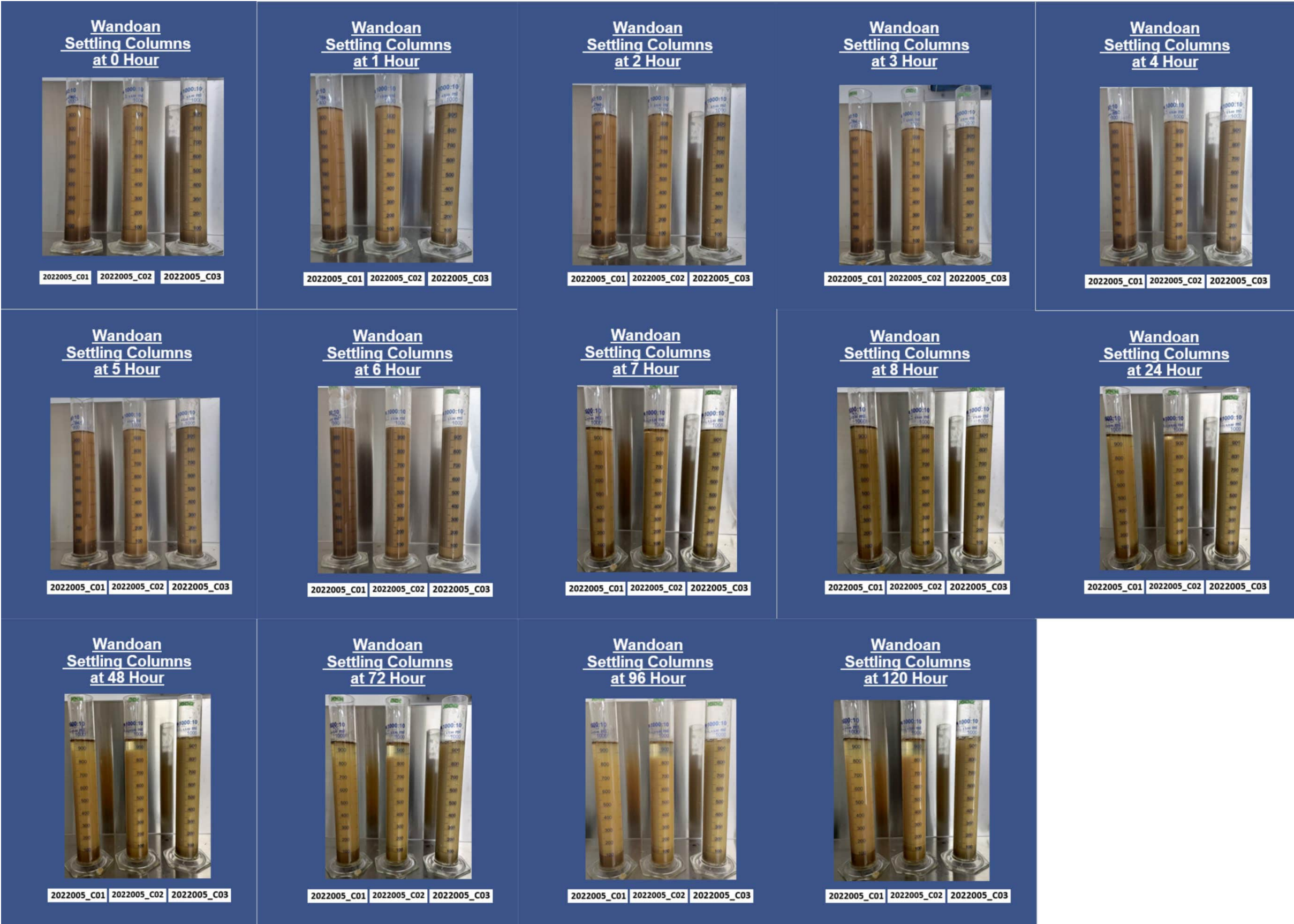
Figure H-1: Column settlement photographs for topsoil and subsoil
