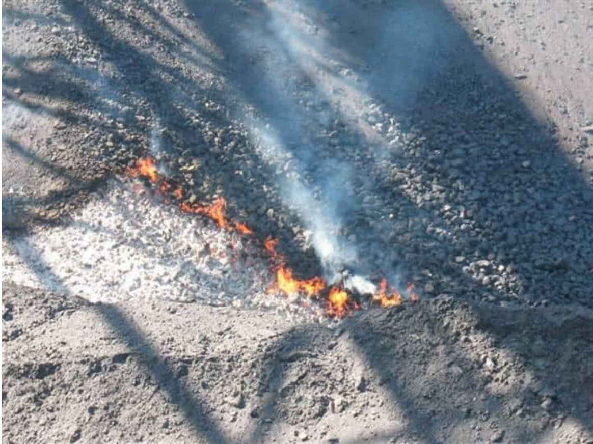
Figure 4. Coal heating developed in uncompact stockpile with steep sides (angle of repose) and coarse coal fraction accumulated at the base of the stockpile allowing pathways for air to enter the stockpile and create a chimney effect. The hotspot has migrated from inside the stockpile to daylight on the surface and reach ignition.
