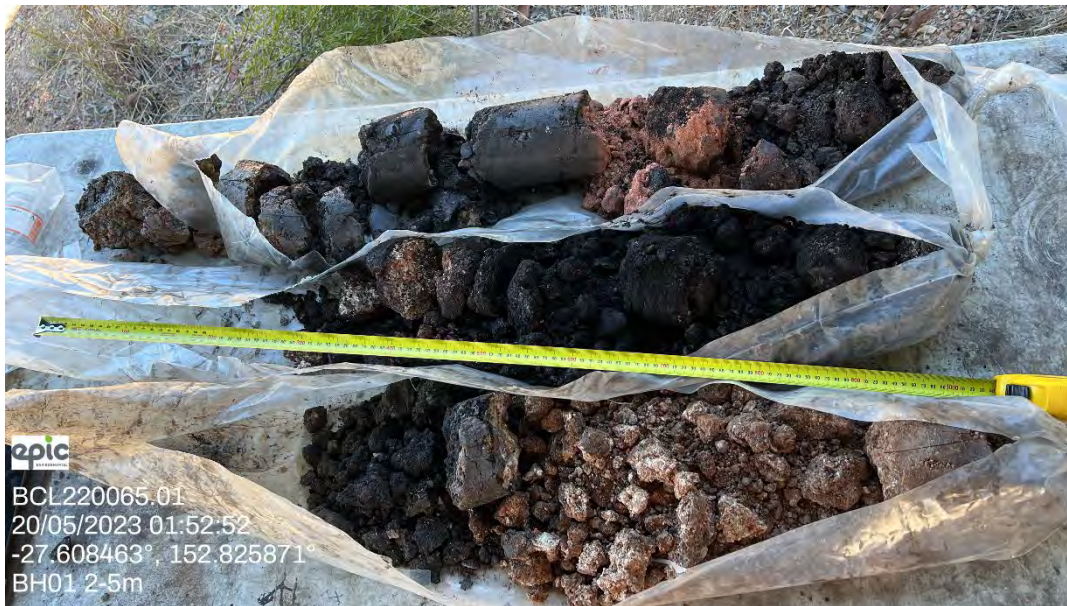
Plate 14. Example fill profile (BH01)
