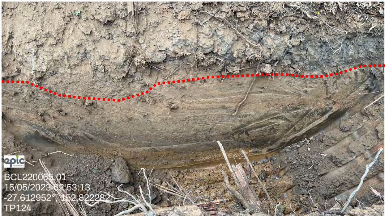
Plate 16. Interface between overburden fill and natural (TP124)
