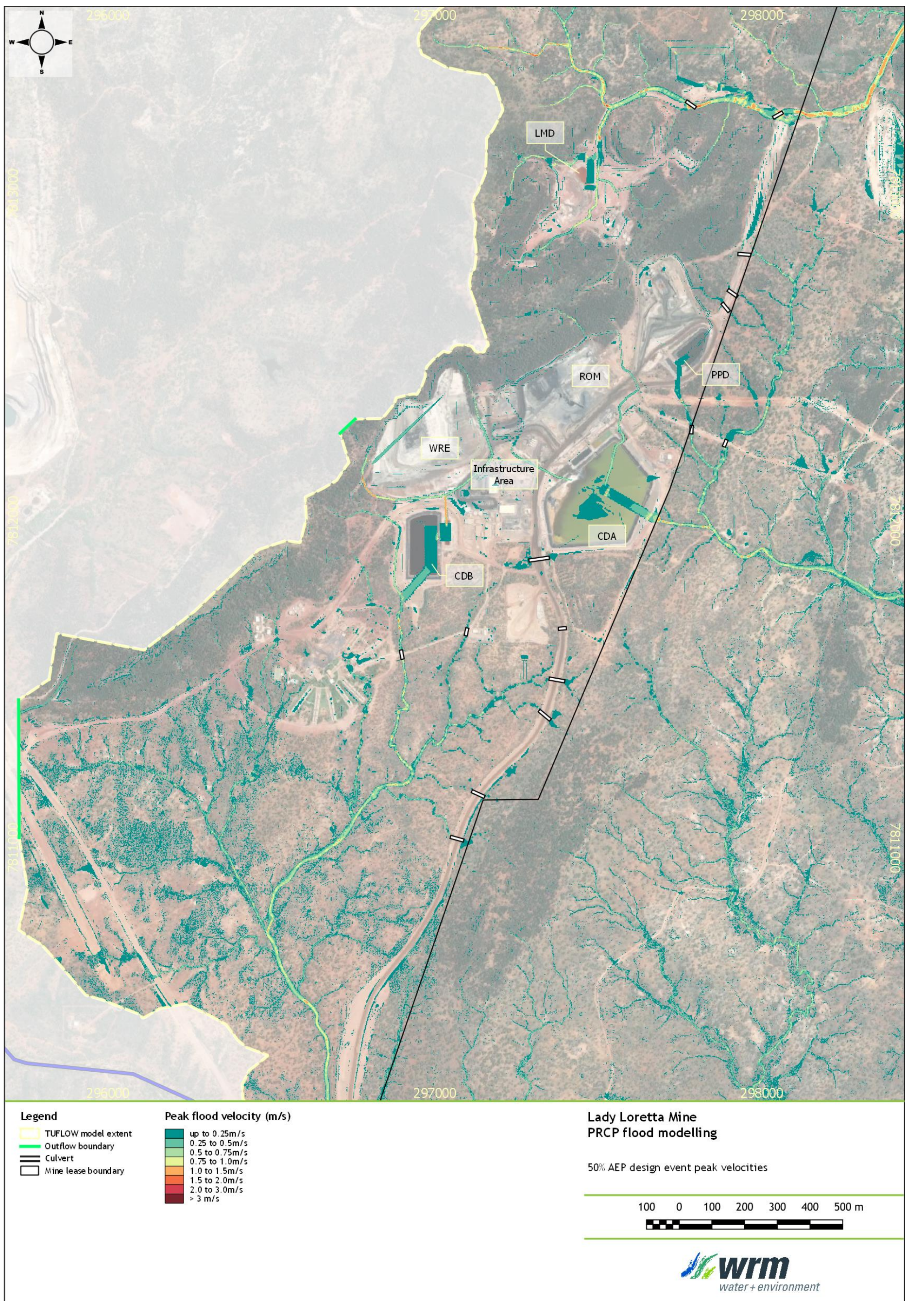
Figure 7.2 - Predicted 50% AEP peak flood velocities in the vicinity of the Mine for post-mining conditions
