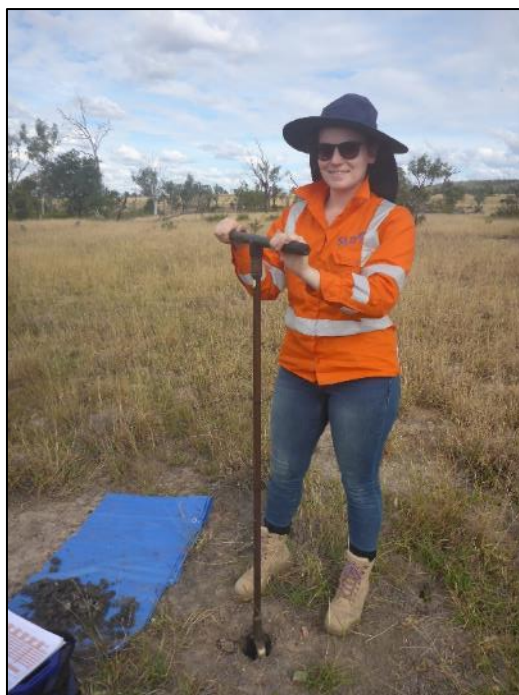
Photo 2 Hand auger used for representative soil profile and shallow subsurface observations
