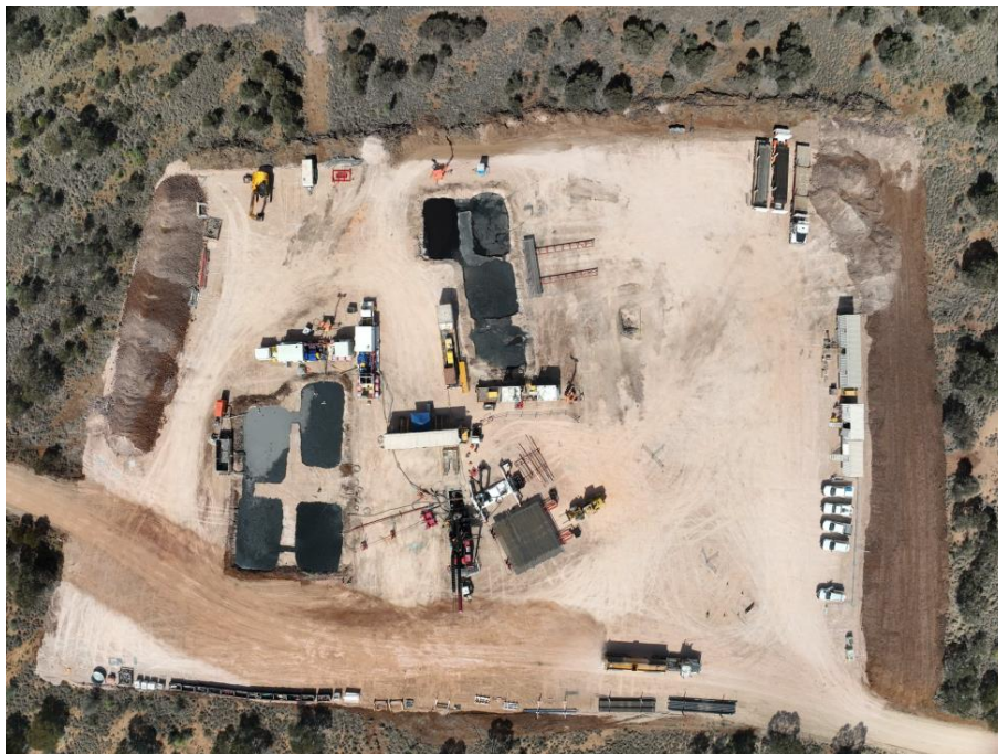
Image 2.2 Example of drill pad arrangement
