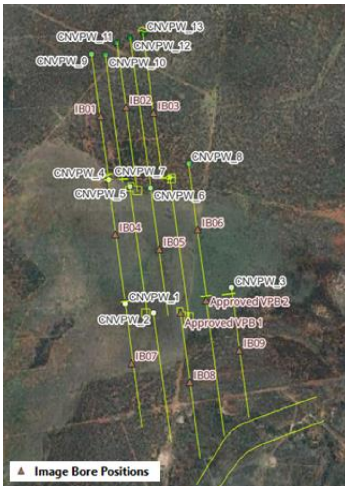
Image 6.7 Bore locations with designed vertical production well collar locations
