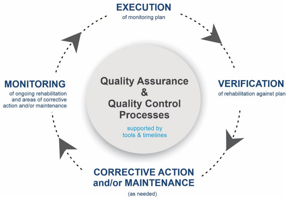
Figure 22 Quality assurance/quality control process to be followed for ongoing rehabilitation monitoring at Centurion North
