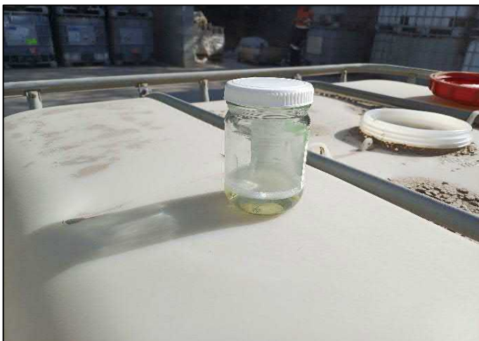
Photograph 1: Example of shake test conducted on IBC water – minimal foaming.
