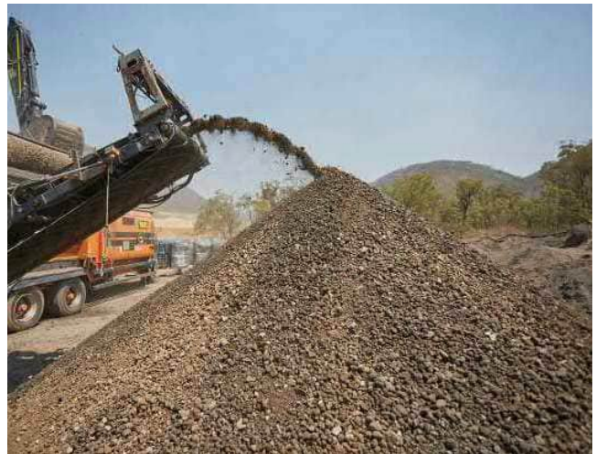
RemBind being applied to treat PFAS soil in Australia
