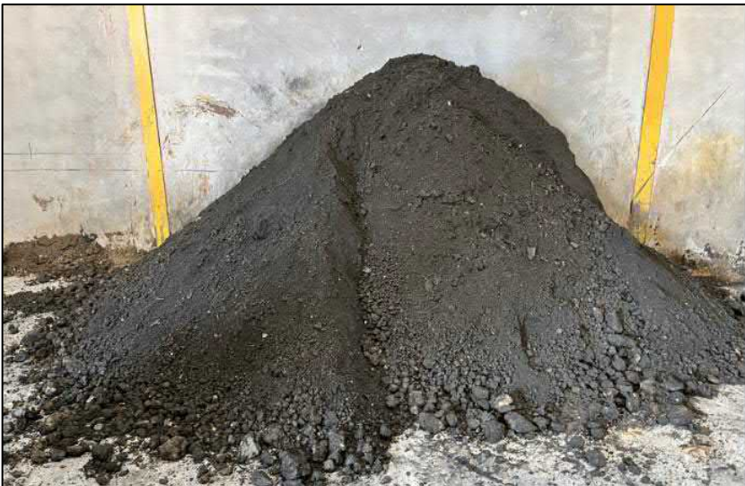
Photograph 12: Batch 3 (Airport soils) following treatment, showing reduction in particle size and homogeneity of material.
