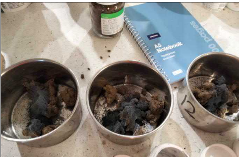
Photograph 5: Mixing of RemBind with clay soils (Bucket 1) for bench trial
